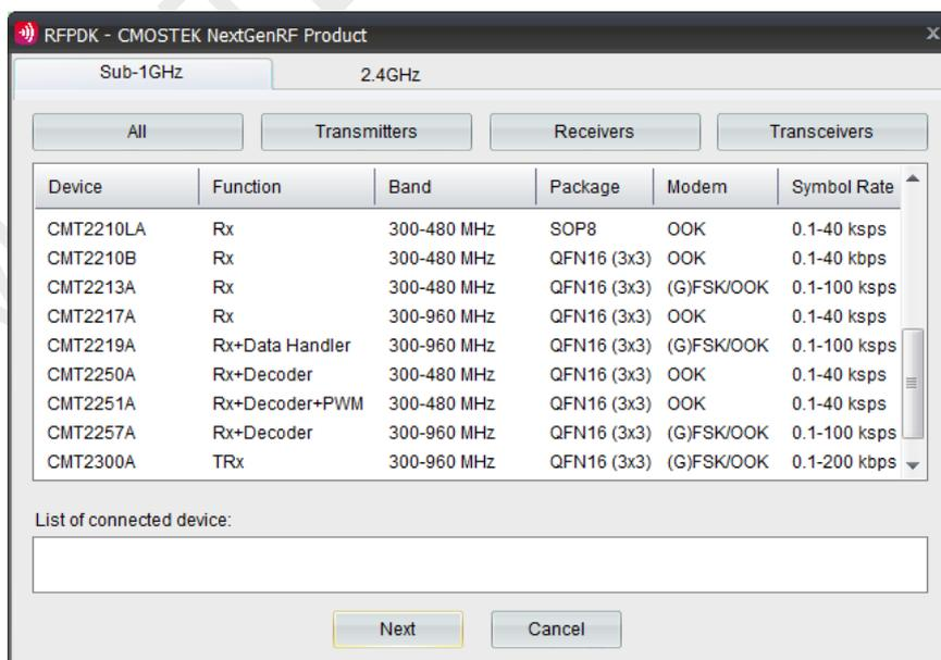
Figure 2. Device Selecting Panel
