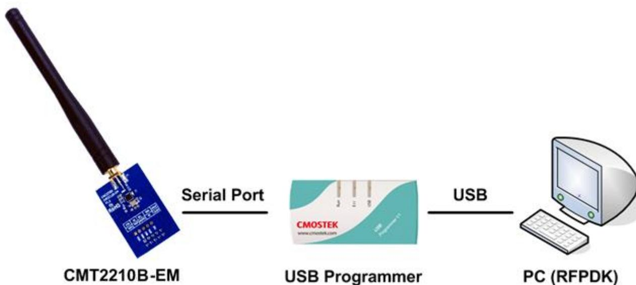
Figure 1. CMT2210B Configuration Setup
